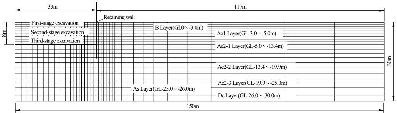
Fig. 2 Finite element meshes
