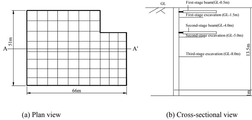
Fig. 1 Configurations of braced excavation
