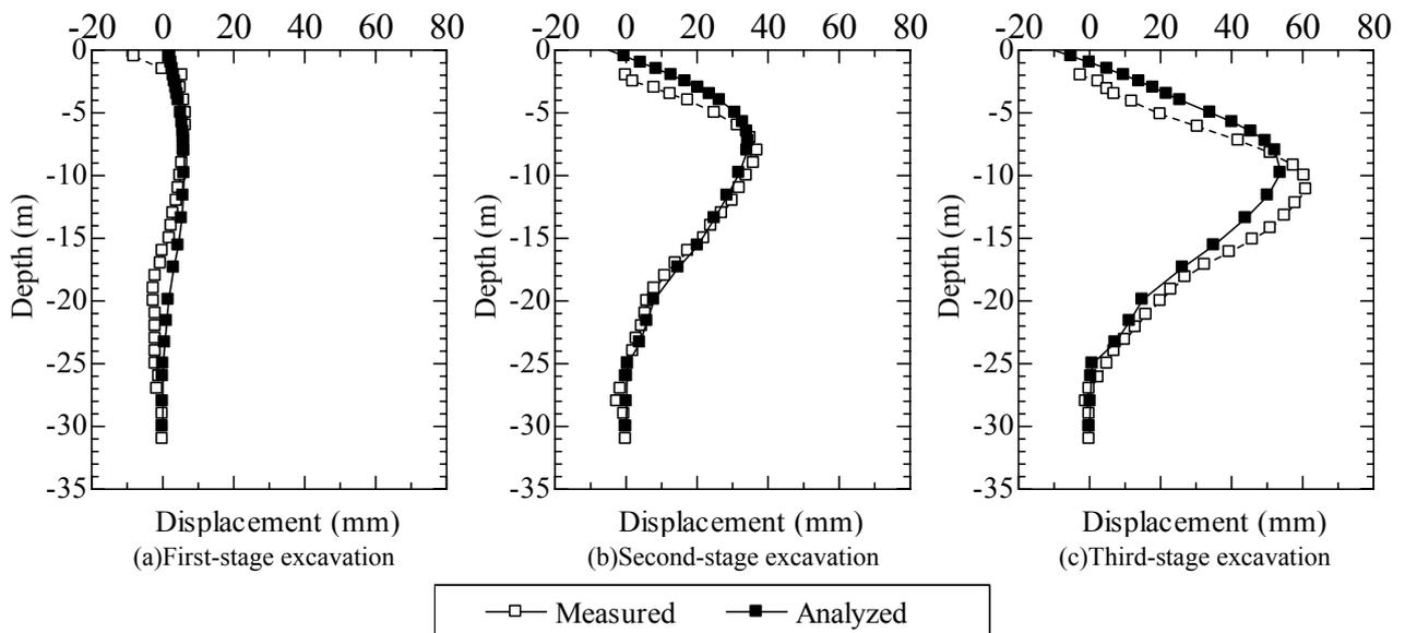
Fig. 4 Displacement of retaining wall (Duncan-Chang model)
