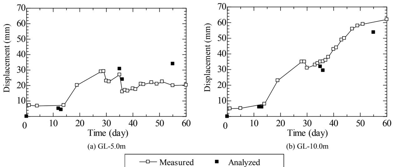
Fig. 6 Variation of displacement of retaining wall (Duncan-Chang model)
