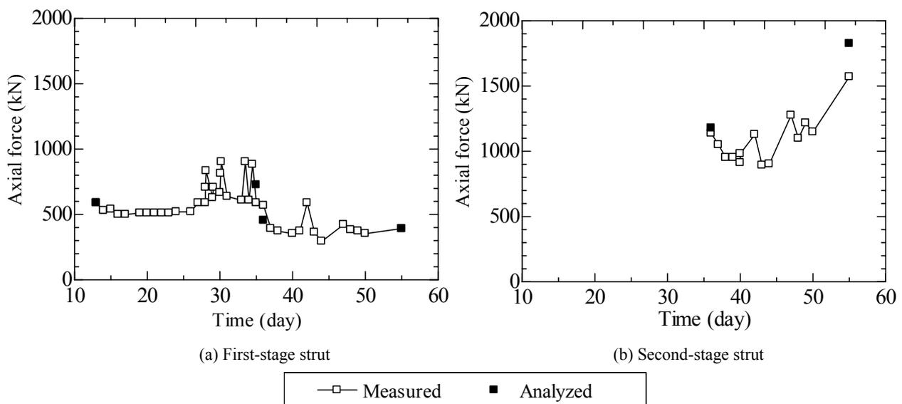
Fig. 8 Axial force of strut (Duncan-Chang model)
