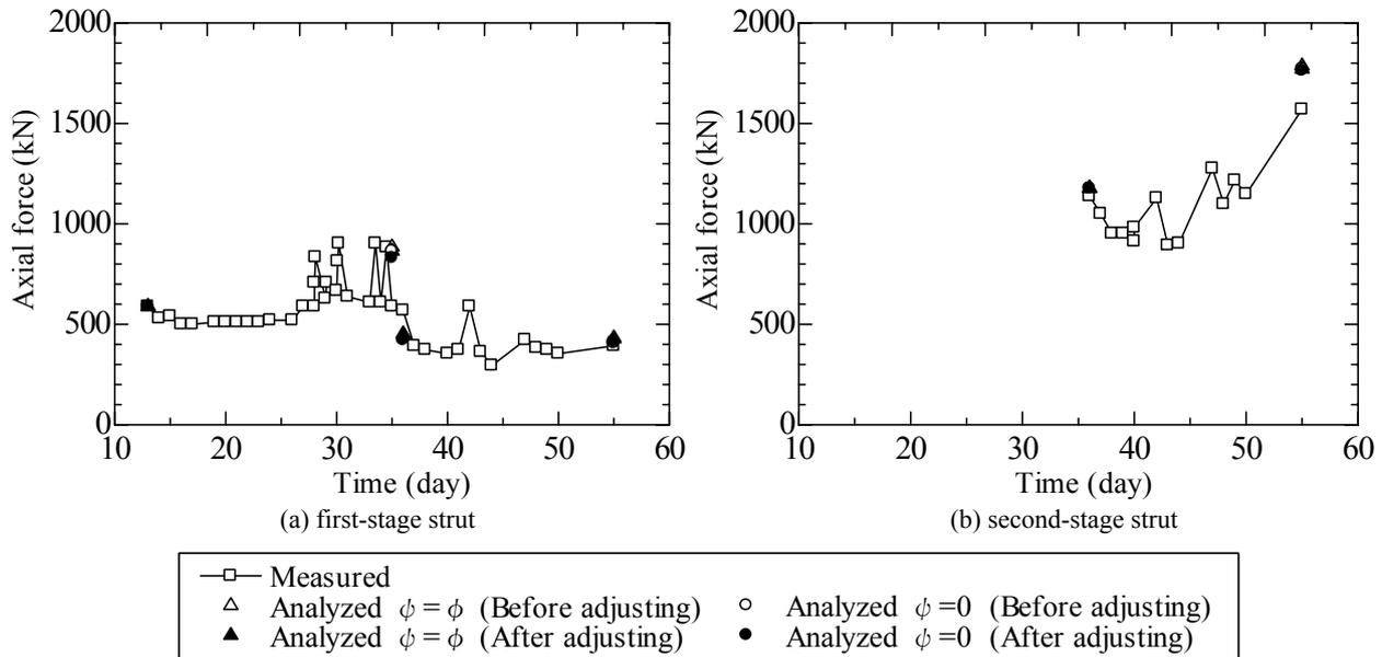
Fig. 7 Axial force of strut (MC-DP model)
