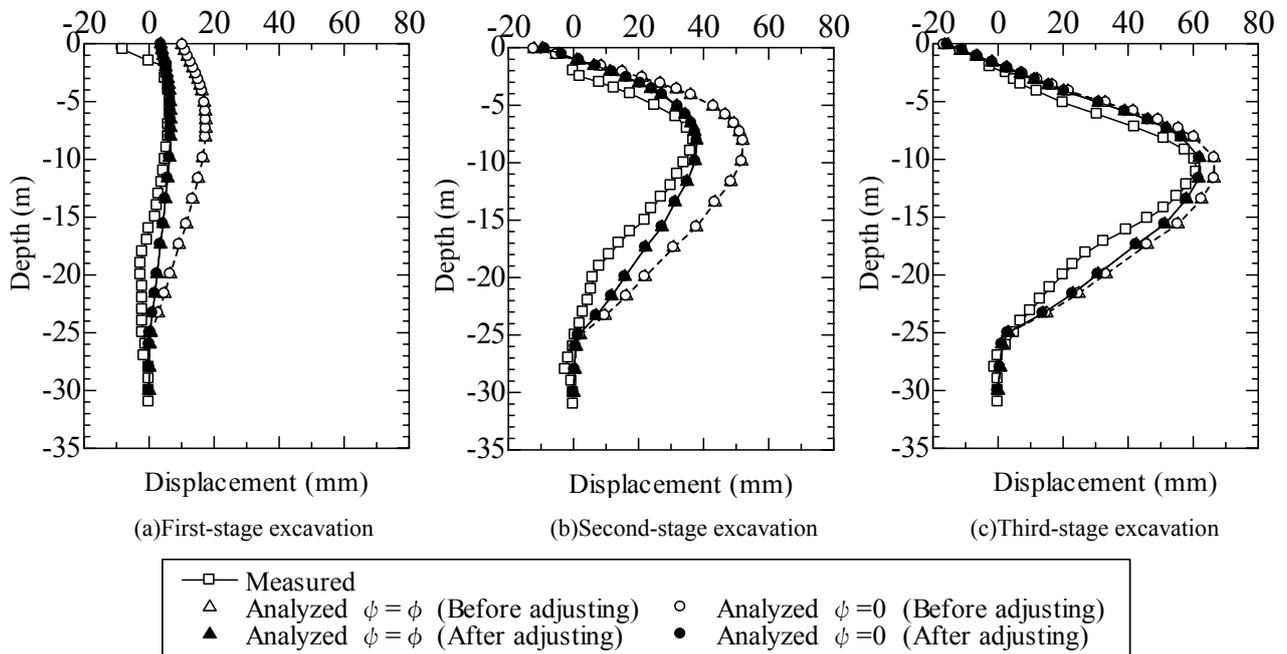
Fig. 3 Displacement of retaining wall (MC-DP model)
