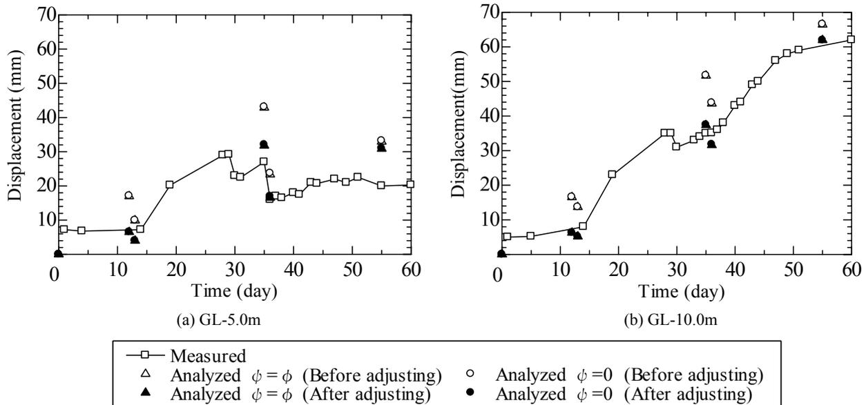
Fig. 5 Variation of displacement of retaining wall (MC-DP model)
