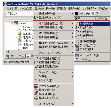
Arrange IP point, and create the following route shape. \*Right-click to finish drawing.
