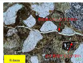
Injected gels into crack gaps
