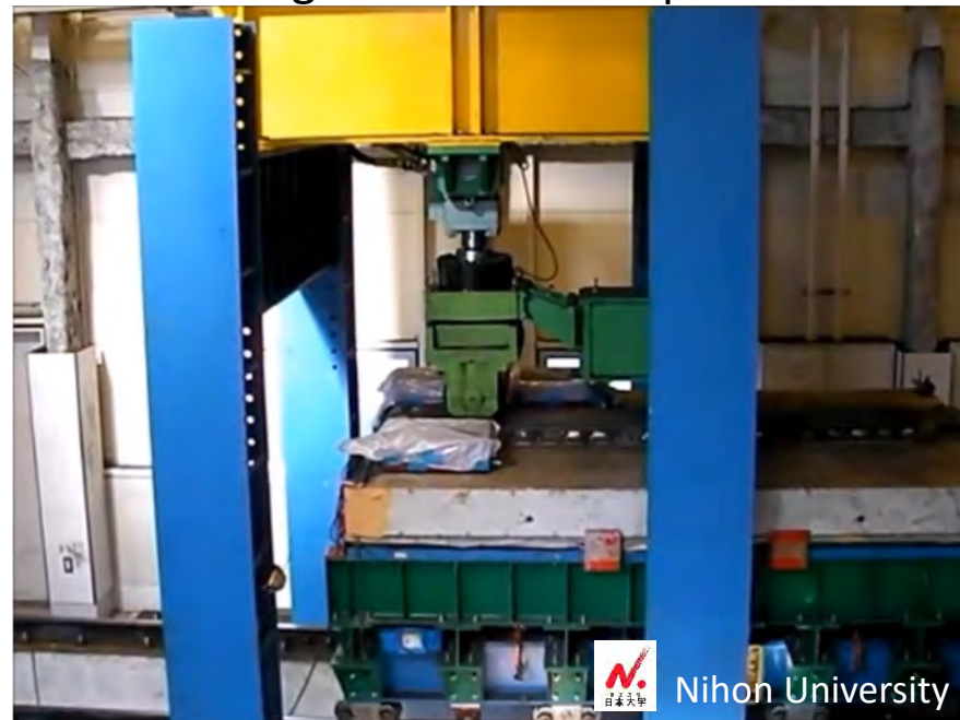
Wheel loading test of RC slab specimen
