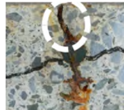
Injected and migrant of corrosion gel through cracks
