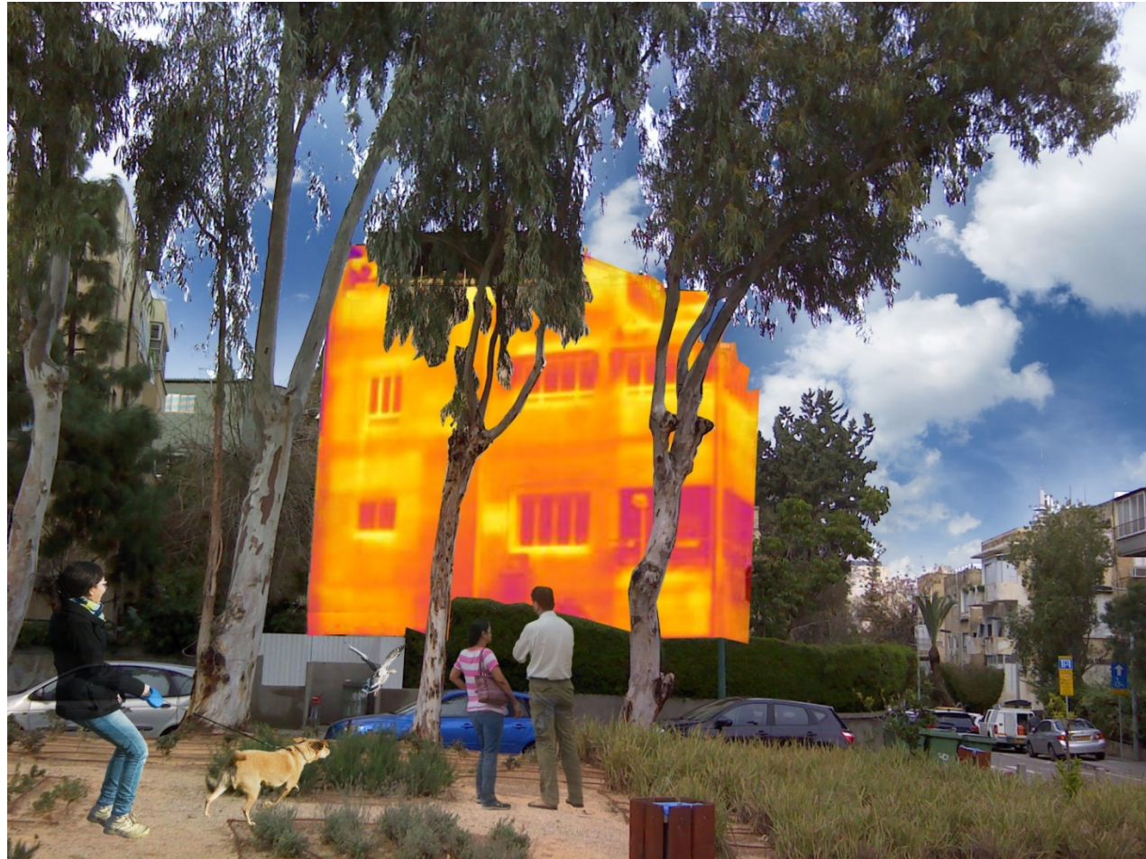
Exposure of a "thermal bridge" from the concrete structure
