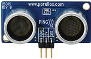
Ultrasonic Sensor: Used to track proximity of people to surface and generate inflection points
